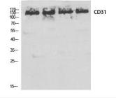
Western blot analysis of lysates from 1) HepG2, 2) K562,3) L929,4) MOUSE-BRAIN cells, (Green) primary antibody was diluted at 1:1000, 4°over night, secondary antibody(cat:RS23920)was diluted at 1:10000, 37° 1hour. (Red) Actin  $\beta$  Monoclonal Antibody(5B7) (cat:YM3028) antibody was diluted at 1:5000 as loading control, 4° over night, secondary antibody(cat:RS23710)was diluted at 1:10000, 37° 1hour.
